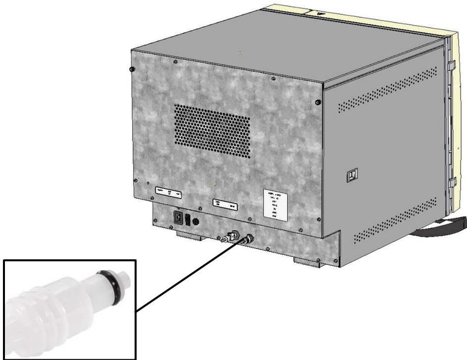
3. Machine will drain into drain container during cycles. Ensure external drain container is emptied regularly between cycles as container could overflow.
