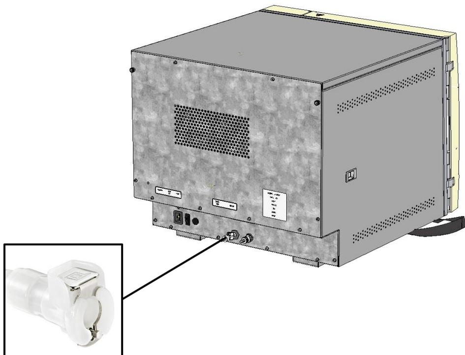
1. Plug Push fit connector into the water fill connector at the rear of the machine, pushing the connector until it “clicks” into position.
