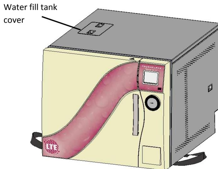
2. Squeeze together latches on the water fill tank cover and remove the cover from the lid.
